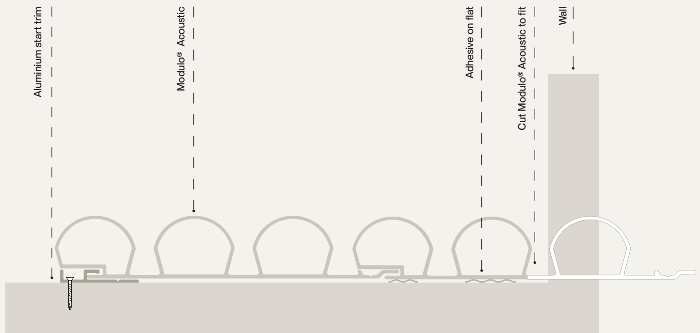
Figure 6. Section view of cuts and adhesive example
