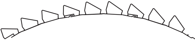
Convex curve 300mm Curve Radius
