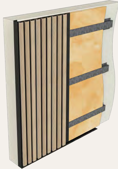
Figure 5. Continue fixing Modulo® Acoustic
