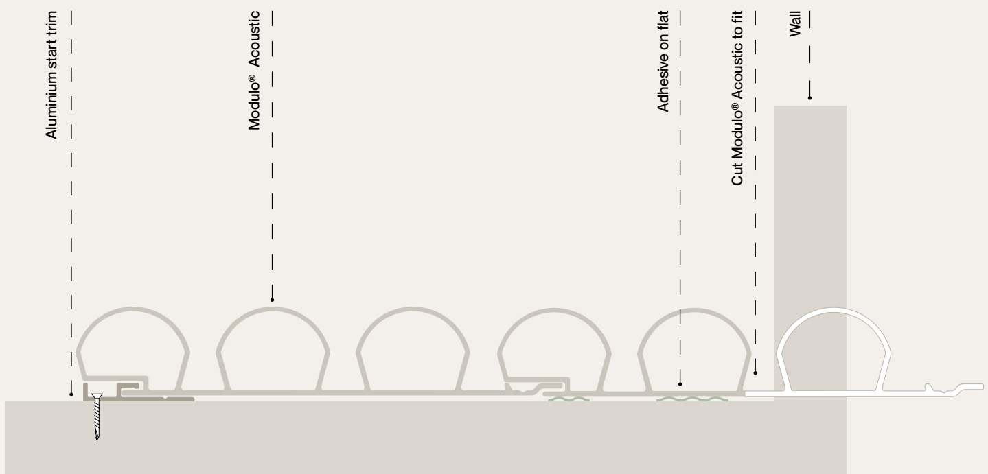
Figure 6. Section view of cuts and adhesive example
