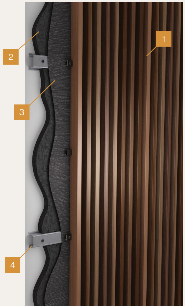
Figure 7. Panels typical acoustic wall installation
