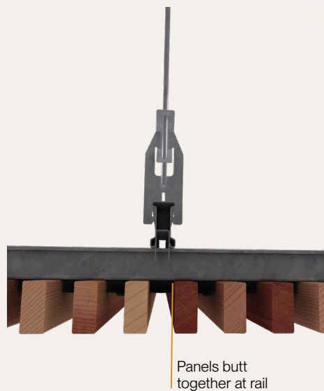
Figure 3. Panels fixed in place
