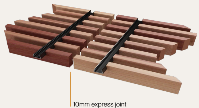
Figure 4. Panels end to end detail
