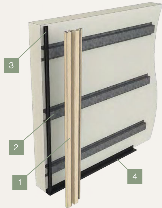
Figure 4. Installing first Modulo® Group 1 panel
