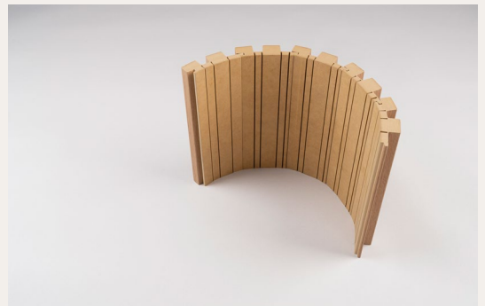
Figure 3. Relief cuts allow the profile to curve
